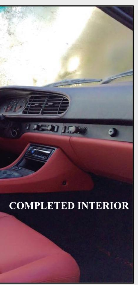
The glove box lid may not line up correctly either, so you will have to trim the leather behind the lid as pointed out previously. Another tip is to trim the vinyl between the dash and the leather where the glove box mounts to the dash. Overall, this was not a very difficult job; it just required a lot of patience and attention to detail. Even with that, I became a victim to hindsight more times than I would have liked. In the end it was a fantastic learning experience with fantastic results.
