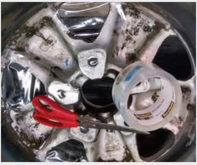
Next up was to pour in the satin black paint (quart can of Rustoleum). I placed the wheel over a plastic container and leveled it out using tapered cedar shingles I happened to have from a previous house project. I also placed several quart paint buckets un-
