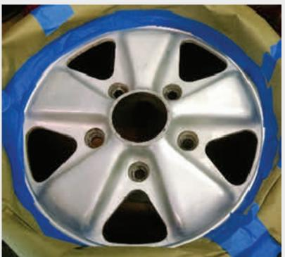
But first I needed to paint the petals with the Dull Aluminum. Since the outer part of the wheel had a decent anodized finish I taped over the area I wanted to remain untouched by paint. I then cleaned again, tacked and painted several coats with the Dull Aluminum spray paint.
