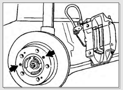
When the pad wears down to the hole, the sensor will from the hydraulic brake system, but will only activate scrape against the rotor and create a short circuit, thus the rear wheels. Not great for breaking, but better than triggering the brake-wear light.
