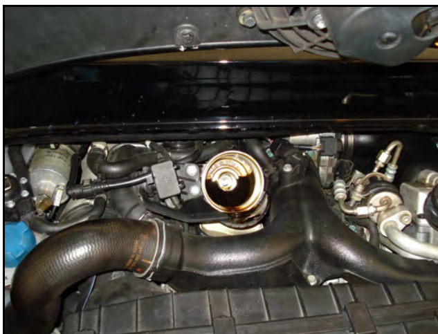
Figure 1. Oil filter has been removed.
