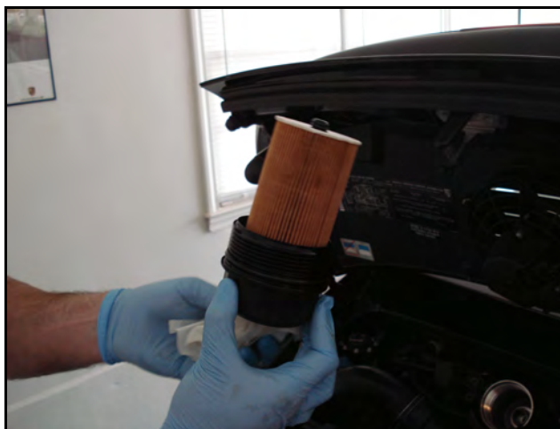
Figure 3. Filter assembly with new filter element.
