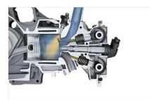
In an internal combustion engine, its compression ratio is a single number that can be used to predict the performance of the engine. It is the ratio between the maximum volume of the combustion chamber and cylinder, when the piston is at the bottom of the stroke and the minimum volume when the piston is at the top of its stroke.
